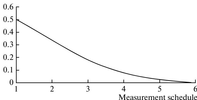
**Fig. 4.** Probability of erroneous proof of the observance of established regulations based on the results of 2 (point 1 on the abscissa axis), 4 (point 2), 12 (point 3), 52 (point 4), and 365 (point 5) measurements and in the case of permanent measurement (point 6).
