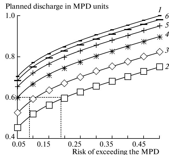
**Fig. 3.** The optimal amount of discharge at  $\sigma = 0.18$  and  $\gamma = 0.95$ . (1–6) The dependence of  $\alpha$  on the measurement frequency at a fixed  $\mu'$ : (1) permanently; (2) semiannually; (3) quarterly; (4) monthly; (5) weekly; (6) daily.
