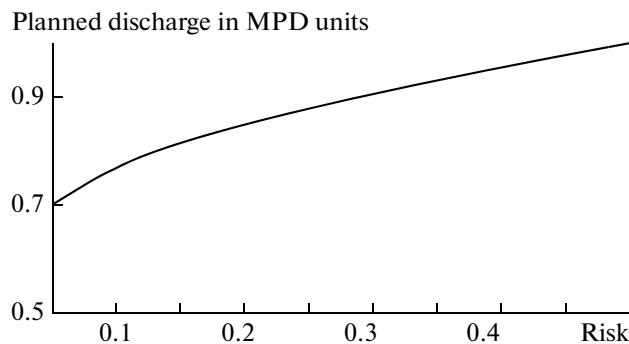
**Fig. 2.** Dependence of the CMD planned by an enterprise (expressed as a proportion of the MPD) on the specified risk within the range 5–50% at  $\sigma = 0.18\mu$ .
